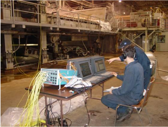
Figure 2: BEL Engineers acquiring multi-channel (128 simultaneous measurements) vibration data
