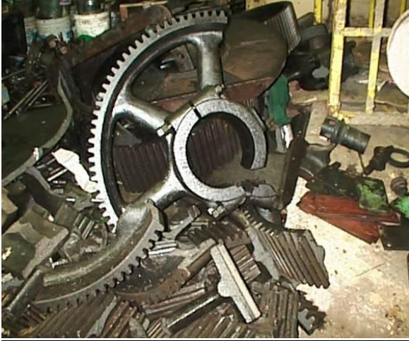
Figure 4: Result of catastrophic failure of a paper machine
